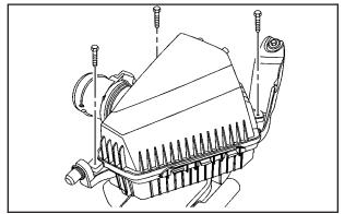
Remove the three air cleaner housing cover screws.
